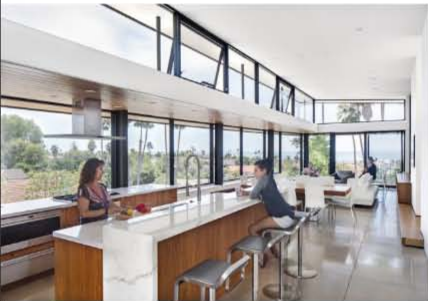
Above: A clerestory light shelf traces around the living space encouraging sunlight to penetrate deeply into the home while softening the strong southern light. Operable windows above help cool the house naturally.
