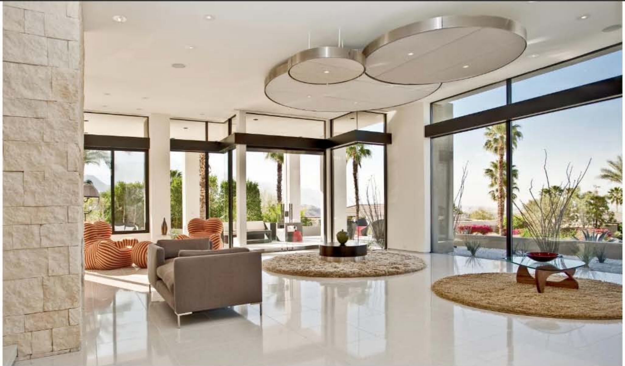
Left: A home's orientation to the sun is primary. In this case, the north-facing windows of this Lasater-designed Palm Springs home invite a generous amount of indirect light deeply into the living space without the direct heat of a harsh southern exposure.
